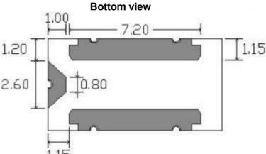
The surface shell is made of LCP material, and the bottom substrate is made of alumina ceramics
