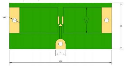
Fuse links are soldered to the prescribed circuit board (Fig 1) with Pb-free solder (Sn96.5/Ag3/Cu0.5 [%]). Covered wires(L=15cm) that provides to Table.1 are soldered to the board's Terminal①,③ by the solder above.
